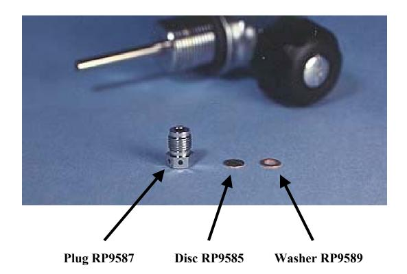
Remove the parts listed, it may be necessary to use a pick to remove the disc and washer. Take care not to damage the threads.
