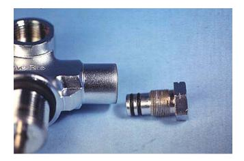
The manifold can be disassembled and the valve posts used on single cylinders by installing a plug Note: The Left hand post has a reverse threaded plug the plug has grooves cut in the edges for identification
