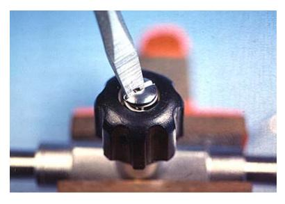
Install and tighten Spring Retaining Nut VA2531 with slotted screwdriver
